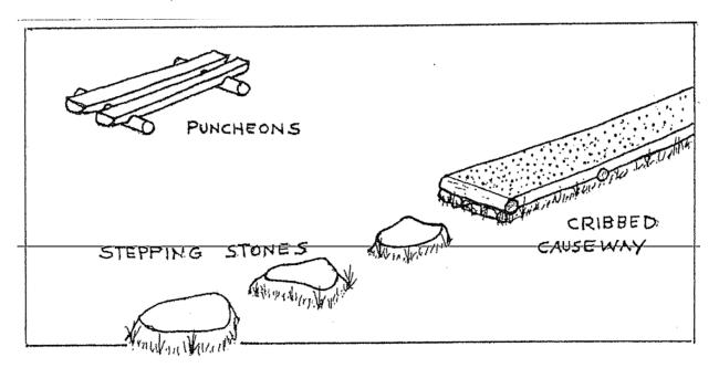
**Stepping stones** are the quickest fix and do an excellent job on short sections of wet trails. Hikers will try to avoid them unless they are properly spaced, large enough to have a solid, stable look and provide an ample flat surface for stepping and do not protrude more than an inch or two above the wetness.
