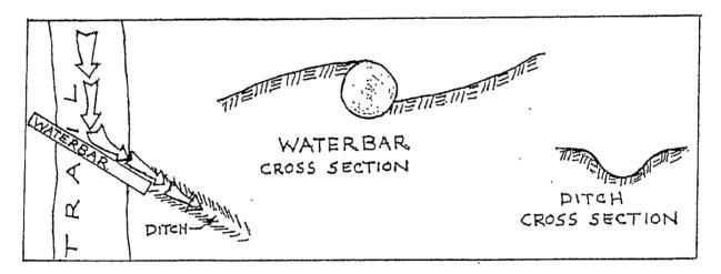
If you take an inventory of all the water bars on your trail you will probably notice that many have at least one deficiency. For some this may be due to poor construction or maintenance but for most it is simply because site constraints limited what could be done. The result is less than perfect but should be the best possible solution for that situation.
